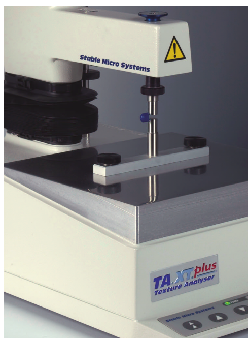
The capsule tensile rig measures the force required to split one half of a hard gel capsule, enabling manufacturers to investigate the effects of fillings on the mechanical strength of the capsule shell. (Source: Stable Micro Systems)
