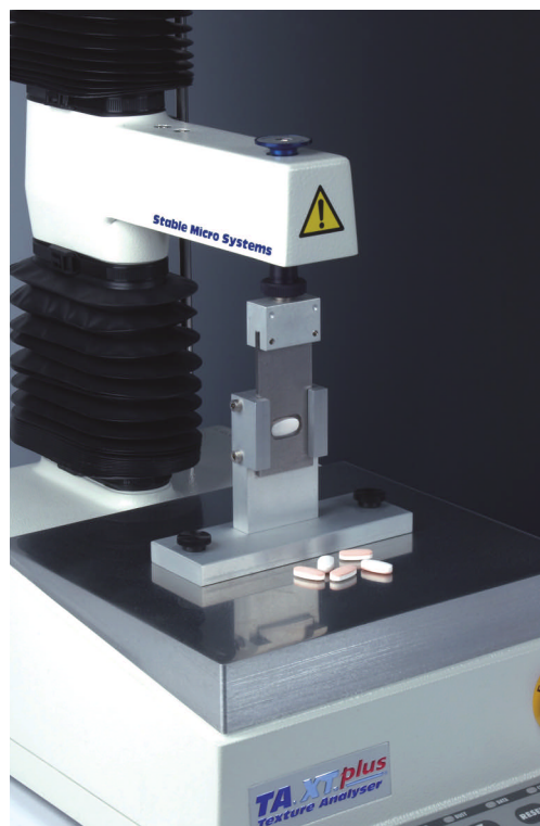
The bilayer tablet shear rig is used to gauge and optimize the stability of tablets which contain isolated immediate and controlled release component layers. (Source: Stable Micro Systems)
